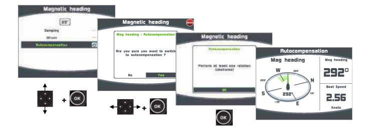
While swinging the *fluxgate*, or *Regatta* compass, you can display the Course Over Ground in a window to show the progress of the manoeuvre. In the case of the *Regatta* compass without COG data on the bus the progression will not be displayed and you will need to follow the procedure from the bowl compass at the helm.
