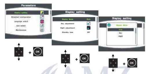
Auto: Backlighting toggles automatically between Night and Day settings, driven by a light sensor. The Backlight intensity and the Skin are those set for each Mode.
