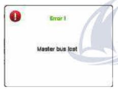
The "master" display is unplugged or out of order. This can be solved by replacing the "master" display by another one. (Refer to "Topline addresses" section).
