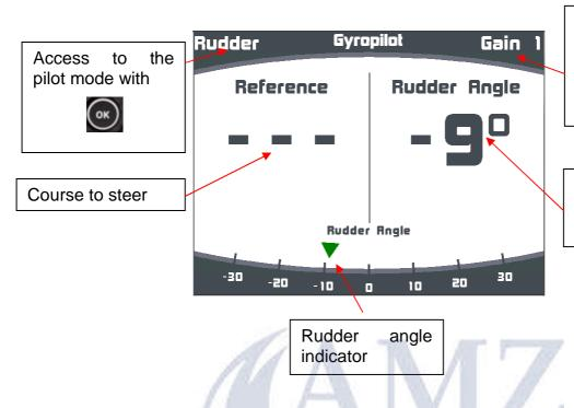
Gain value adjustable with the up and down arrows on the pad
