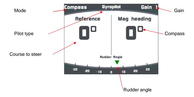
Note: when the pilot is disengaged «---» is displayed instead of the course to steer.
