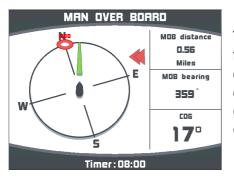
This page is shown when the Man Over Board function has been triggered. The **dead reckoned** distance and bearing to the man over board are displayed together with the boat's course over ground. The timer is triggered to give the time from event.
