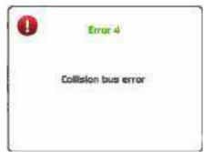
2 similar sensors are connected to the bus and transmit the same data, or an NMEA input has been set for the same data as a sensor present in the bus. Check the connected sensors and reset the NMEA inputs.
