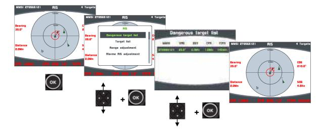
Any target can be selected from the targets list and pressing displays it on the A.I.S. page.
