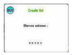
Multigraphic being set as "Master", when the system creates the list (search all sensors and displays in the bus), it displays addresses for slave displays.
