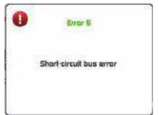
The black wire of the Topline bus cable, carrying the data is in short-circuit with one of the 2 other wires. This can happen in a junction box, the cable itself or one of the units connected to the bus.
