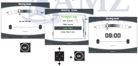
A press on "OK" starts the count-down. A second press on "OK" resets the timer on T2.
